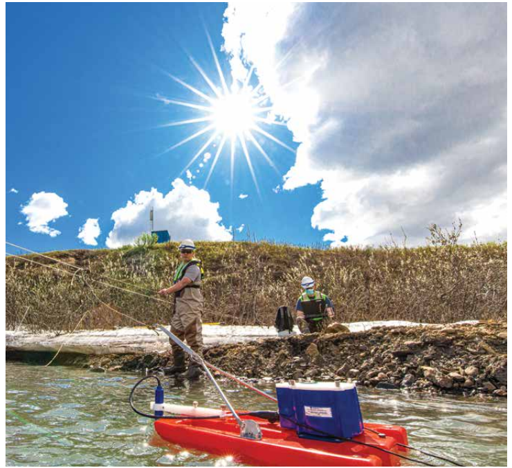
Environmental Technicians Tristen Pattee and Trevor Phillips used a doppler to measure the water flow this past summer.
